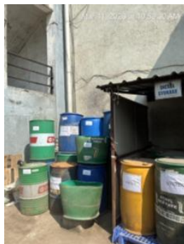
Secondary containment not provided to Diesel & used drums.JPG
